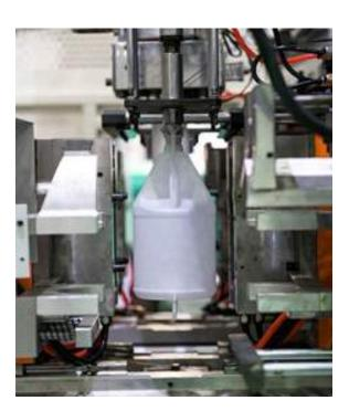
Extrusion blow moulding In extrusion blow moulding, plastic is continuously melted, extruded through a shaping nozzle to form a tube, which is then brought into shape in a mold and cooled down. Multilayer or co-extrusion blow molding enables the production of hollow bodies with a multi-layer wall structure (up to 6 layers. Extrusion blow molding allows the efficient production of containers with volumes ranging from 5 ml (eye drop ampoules) to 5,000 ml (canisters) in smaller quantities.
